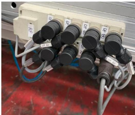
An additional advantage of routing cables through the inside of tubes and profiles is the reduction of the assembly time: it is no longer necessary to fasten each cable and tube with Velcro and screws.
